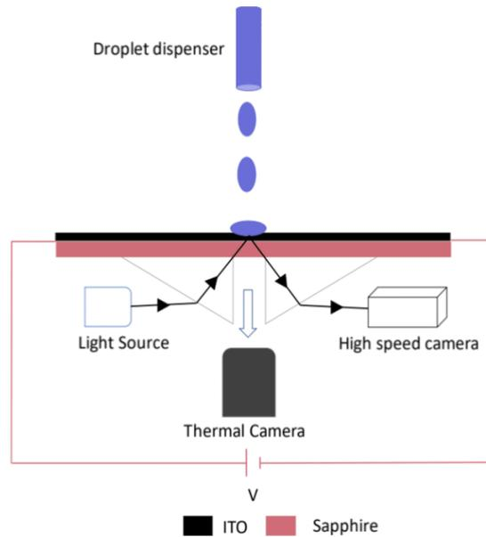
**Figure 1.** Schematics of experimental setup for capturing the geometry evolution of droplets impinging on superheated surfaces. Thermal camera underneath allowed us to capture the thermal footprint of droplets on ITO surface. Total internal reflection imaging (added to the setup, results not presented here) would help us determining whether droplets contact the surface or not.
