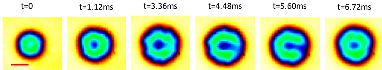
**Figure 3.** Temporal evolution of complex droplet geometry upon impact on superheated surfaces. Scale bar equals 1mm.
