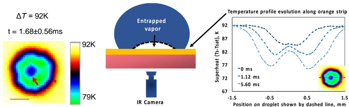
**Figure 2.** Thermal footprint of droplet impinging on heated substrate captured using an infrared camera underneath. The temperature profile along diameter of thermal footprint is shown for three time instances. Scale bar equals 1mm.
